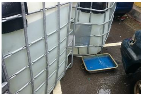
IBC桶傾倒破損
